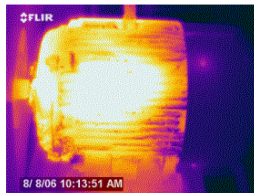
Above thermal and daylight images show a three phase motor which has overheated. Power quality analysis proved condition was caused by negative sequence harmonics.
